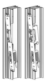
**7.** Screw to adjust the switching point partially with hex key, size 2.5 mm. Unscrew or completely remove.
